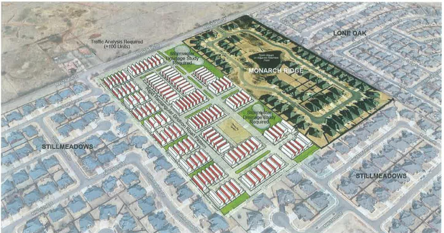
Red indicates where Structure sits directly on Property Line and is thus subject to IRC 2015 Table R302.1(1) Exterior Wall Fire Rated Assemblies and No Projections or Openings Allowed
